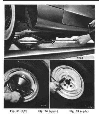
Wheel Changing Procedure (Pressed Steel Wheels)
